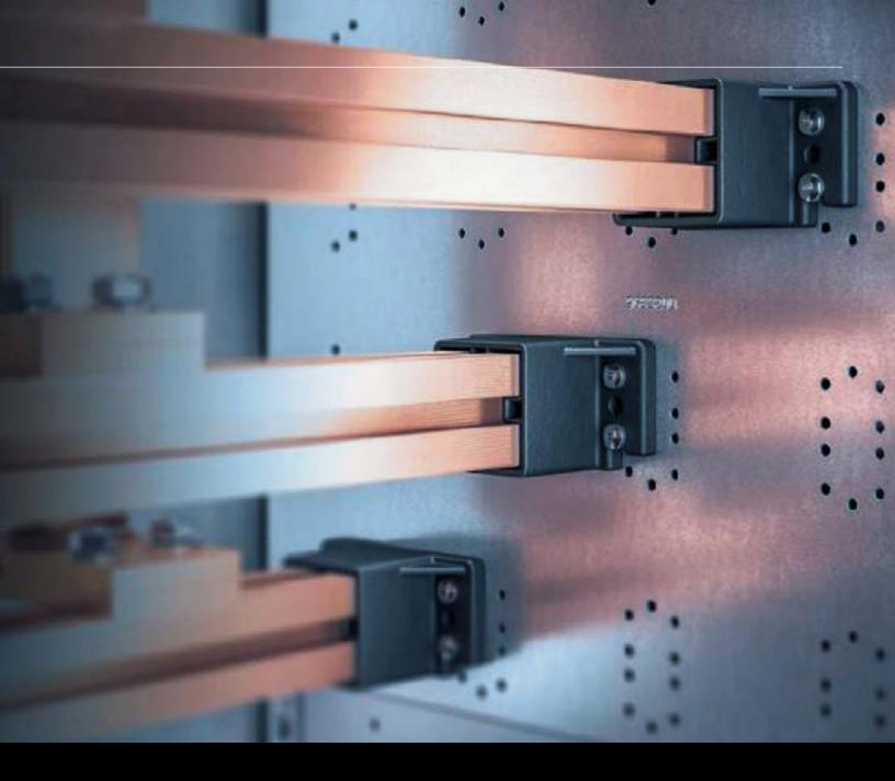
Rittal busbar supports fit dimensions from  $40 \times 10$  mm to  $120 \times 10$  mm. The support may be top-mounted with components using the pitch pattern of the cover system. In addition, Rittal meets and exceeds power demands to withstand current ICW up to 50kA, with rated currents up to 1600 A. All are UL and ETL Listed. Rittal is also the world's first manufacturer to offer an approved busbar system with standard components optimized for both AC and DC applications for international use.
